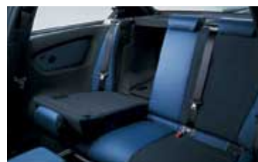
■ Rear seat back, foldable, with asymmetric subdivision (2:1), enables variable extension of the luggage compartment to transport bulky items.
