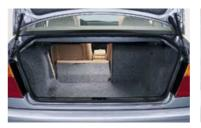
■ Through-loading system: In combination with the asymmetric subdivision of foldable rear seat back (2:1), the through-loading system allows for easy transport of bulky or longer items.
