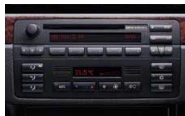
□ BMW Professional: 4 x 20 W power output, 2-tuner frequency diversity (2 tuners constantly search for the best reception and switch inaudibly to the best frequency), integrated CD drive, automatic CD insert/eject, connection for BMW CD changer.
