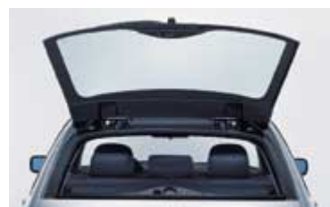
■ Rear window opening separately for rapidly taking out or putting in odds and ends.
